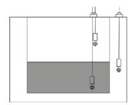
The probe wired to the <u>HIGH</u> connection is positioned at the topmost part of the tank and is used to alert that an overfill has occurred. The probe wired to the <u>LOW</u> connection should be positioned near the bottom of the tank to indicate a low-level. The <u>BUND</u> probe is placed between the two tank 'skins' and is used to quickly alert of any leaks.
